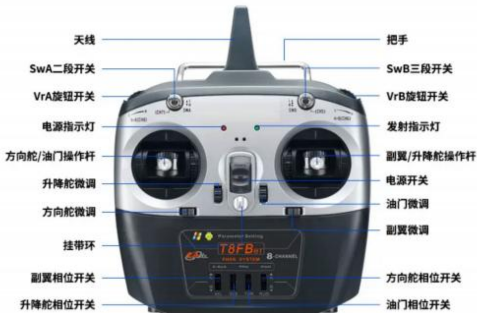
Figure 2 Schematic Diagram of Remote Controller Switch
