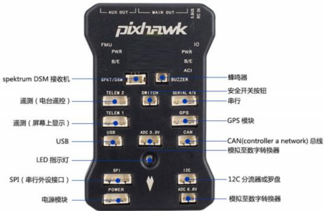
Figure 1 PIXHAWK 2.4.8 Interface Description
